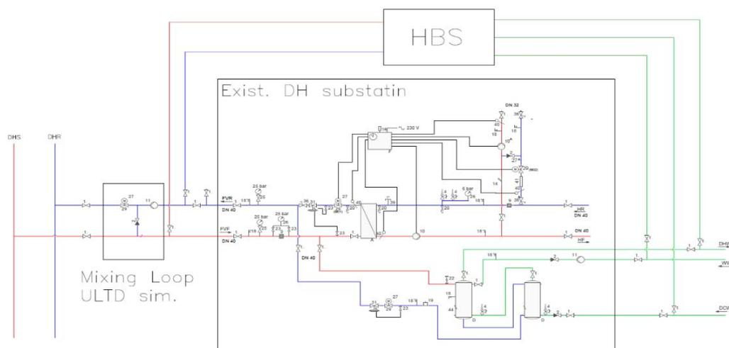
existing DHW system of the building. The existing space heating system was operated in the common way, but also supplied by ULTDH. For the sake of obtaining field experience, the ULTDH was established by a mixing loop, see figure above.
